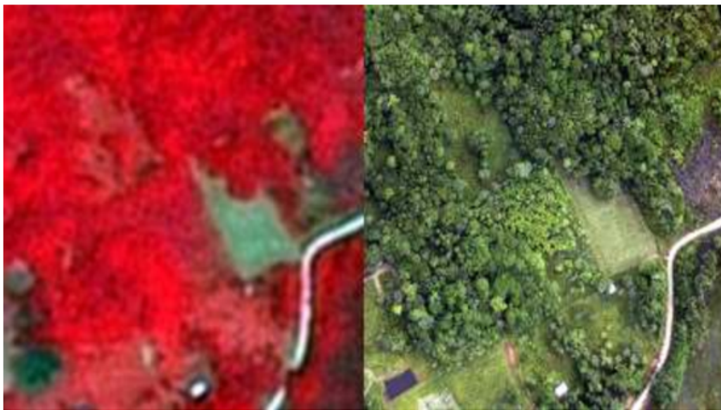
Figure 1: Differences of canopy grain perception between two 300 m 2 subset images of different spatial resolution over a mixed savanna forest-inhabited area, French Guiana. Left: SPOT5 Fusion satellite image acquired in October 2010 (nominal resolution of 2.5-m, larger pixels actually). Right: a 20-cm pixels aerial photograph acquired in July 2010 (L’Avion Jaune). Drone now allows the acquisition of images having similar characteristics.
